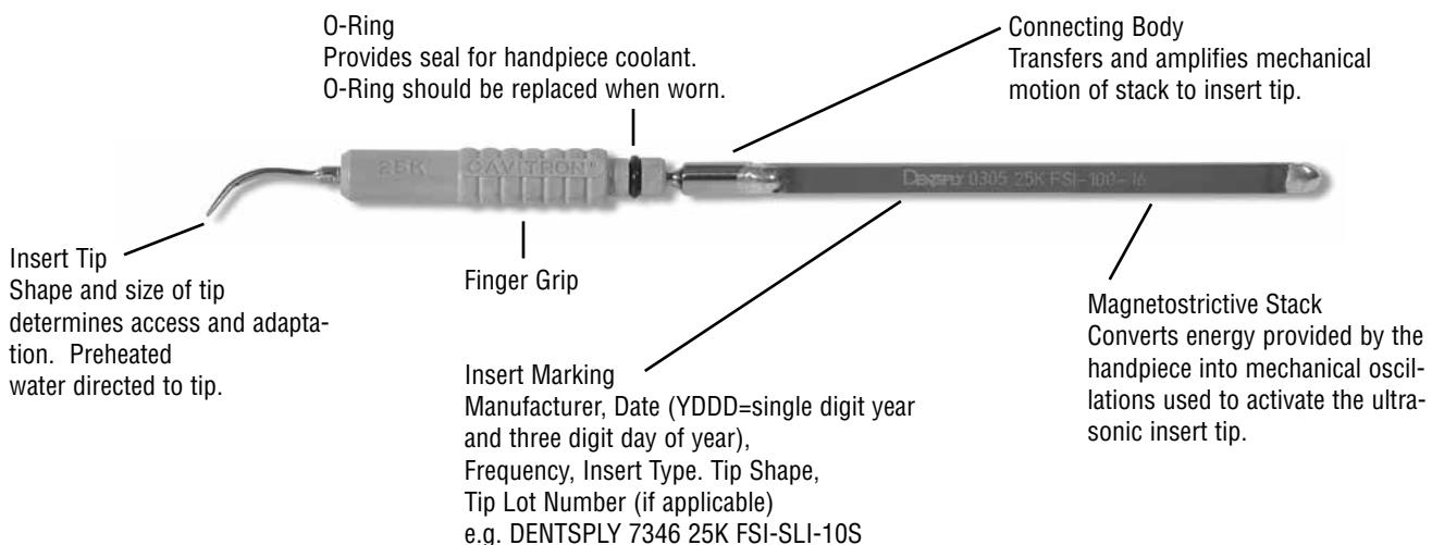
Hold the handpiece in an upright position. Activate the foot control to bleed with water any air bubbles that might be trapped inside the handpiece. Lubricate the rubber o-ring on the insert with water before placing it into the handpiece. Fully seat insert with a gentle push-twist motion. DO NOT FORCE.
