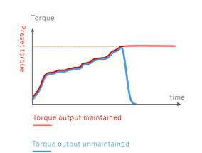
When the torque reaches the preset value, it will continue to output without automatic stop, avoiding insufficient torque output.
